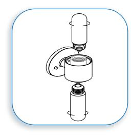
INSERT THE BULBS Insert the bulbs. MAXIMUM WATTAGE 60W. DO NOT EXCEED THE WATTAGE AS STATED ON THE WARNING LABEL AND IN THE INSTRUCTION SHEETS
